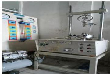
Gambar 4. Alat Uji Triaxial
