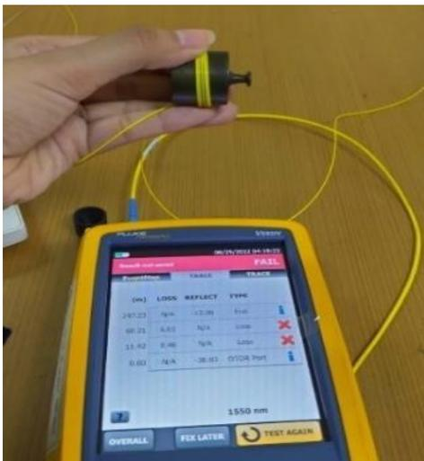
Gambar 2. Proses pengukuran *bending loss*
