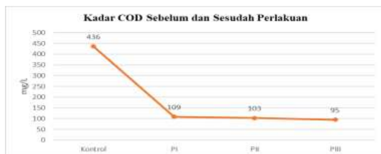
Figure 2 COD levels before and after treatment
