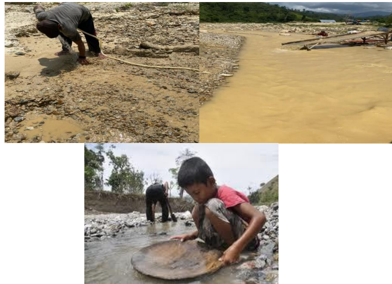
Figure 3. Mining activities using the spray and pan method (Source: Herlindah Documentation, 2023)
