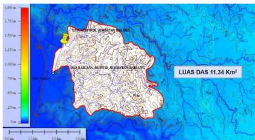
Picture3. Bailang Watershed at Bailang Bridge Point Source: Global Mapper, BWSS-I GIS Data
