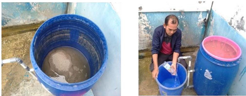
Figure 1. Appearance of the screening tank and slow sand filtering process
